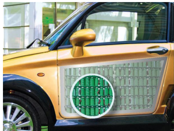
Fig 5: Distributed energy storage concept for vehicles.
